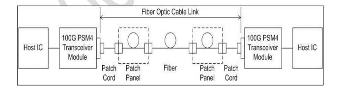
Figure 7: Fiber optic cabling model
