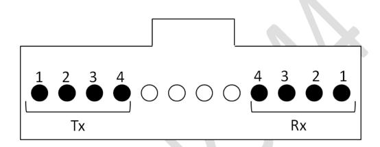
Figure 8: 12 fiber MPO optical lane assignments (looking into module optical port (MDI))
