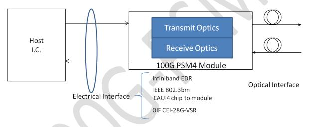
Figure 1: PSM4 system block diagram
