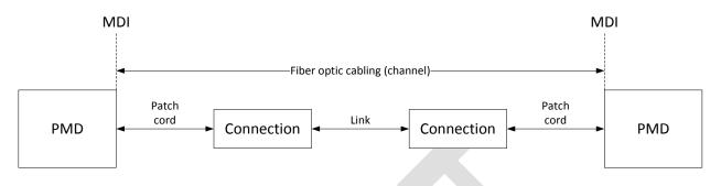
Figure 4-1: Fiber optic cabling model
