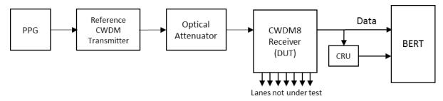
Figure 3: Test setup for receiver sensitivity
