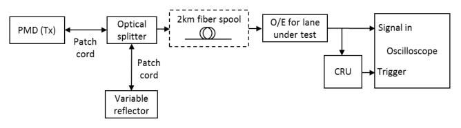
Figure 2: TDEC conformance test setup
