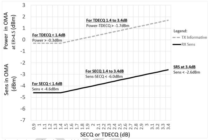
Figure 2-1: Stressed receiver sensitivity mask for 400G-FR4
