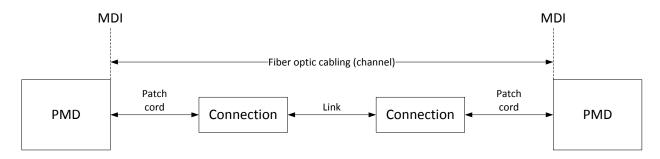
Figure 4-1: Fiber optic cabling model
