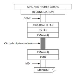
Figure 1-2: Example FEC implemented with PMD
