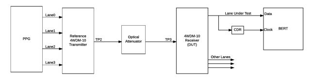
Figure 3-1: Test setup for measurement of receiver sensitivity
