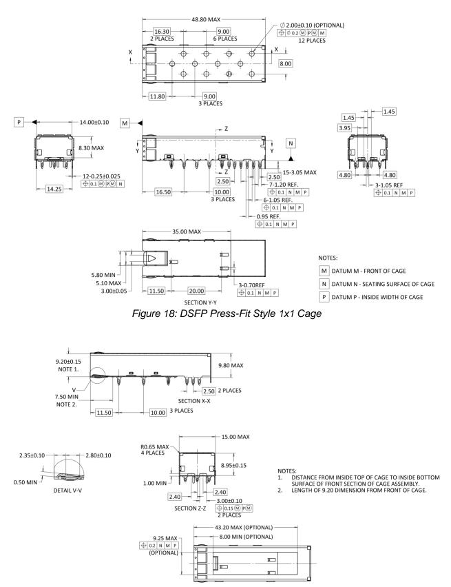
Figure 19: DSFP Cage Latch and Riding Heatsink Details
