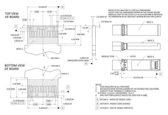
Figure 20: DSFP Module Card Edge and Mechanical
