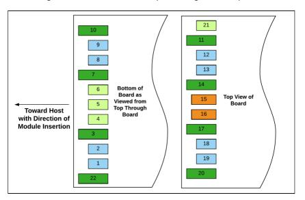
Figure 8: DSFP module contact assignment
