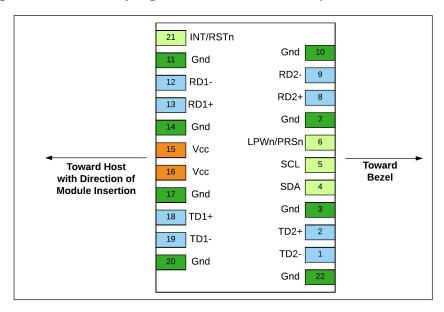
Figure 7: DSFP Host PCB pad assignment top view
