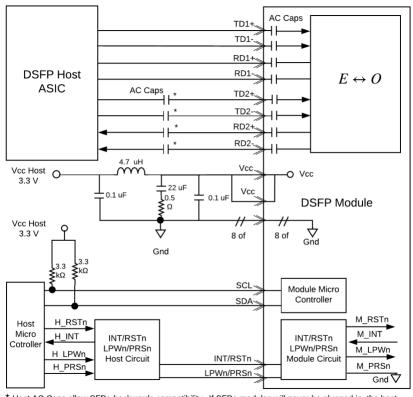
\* Host AC Caps allow SFP+ backwards compatibility. If SFP+ modules will never be plugged in, the host AC Caps can be omitted.
