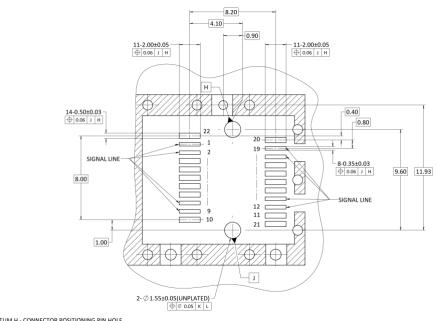
H DATUM H - CONNECTOR POSITIONING PIN HOLE
