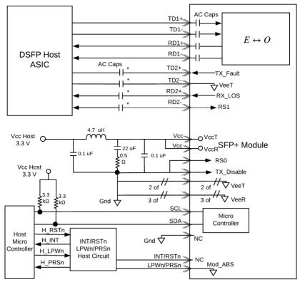
\* A di-plexer that doesn't degrade SI can replace the AC Caps to tap LVTTL signals.
