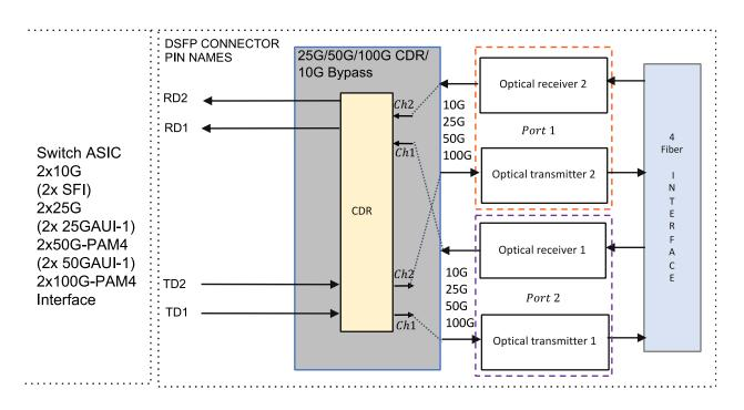
Figure 1: Block diagram for 10/25GBASE-SR/LR or 50GBASE-SR/FR/LR
