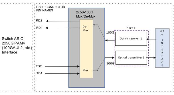
Figure 4: Block diagram for 100GBASE-DR
