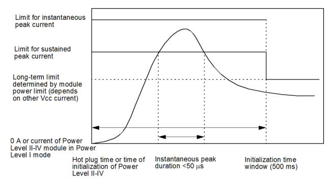
Figure 13: Instantaneous and sustained peak current for Vcc
