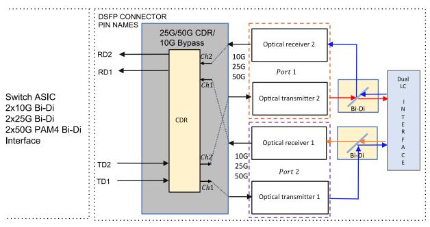
Figure 5: Block diagram for 10G/25G-NRZ and 50G-PAM4 Bi-Di
