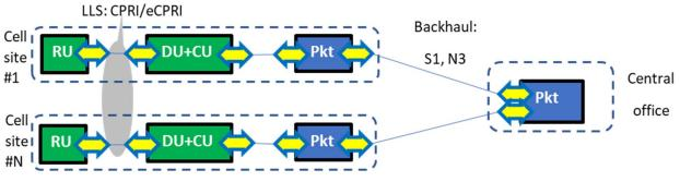
Figure 7: DRAN architecture with RAN nodes, transport nodes and optical pluggables.
