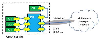
Figure 28: 40 km CRAN hub site backhaul direct parallel fiber Blueprint. The link specified has a gray background. In cases where the CU is located at another location, HLS is illustrated. The pluggables at the CRAN hub site may be C-temp as indicated by dashed borders for the intraoffice ones.
