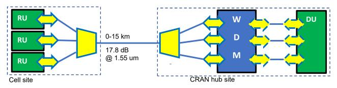
Figure 17: 15 km RU-DU semi-active wavelength multiplexed, P2P or P2MP Blueprint. The intraoffice pluggables at the hub site may be C-temp as indicated by dashed borders.
