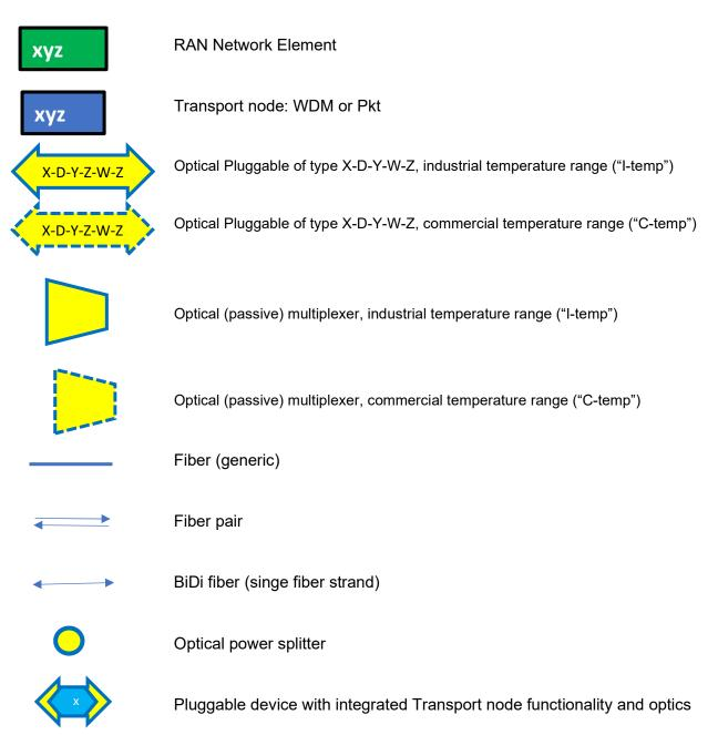
The optical pluggable *type* in the icons above is meant to provide an indication at a glance of the category to which the transceiver belongs. It is meant to be a compact and not allencompassing description: detailed characteristics are provided in the optical Blueprints description in sections 7-9. The semantic of the different type fields is reported in Table 1.
