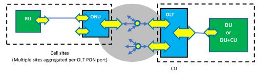
Figure 32: LLS using TDM-PON with separate ONU box.
