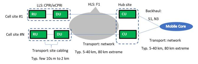
Figure 6: Virtual RAN architecture. The HLS links are highlighted by the gray oval.
