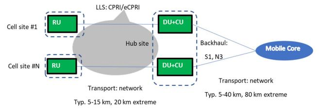
Figure 5: CRAN architecture. The LLS links are highlighted by the gray oval.
