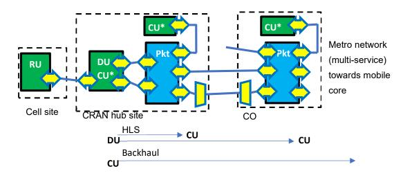
Figure 21: Backhaul and HLS for CRAN. CU\* indicates possible locations for the CU, at the CRAN hub site, or at the CO. The latter constitutes the VRAN case. The pluggables at the CRAN hub and CO sites may be C-temp as indicated by dashed borders for the intraoffice ones.
