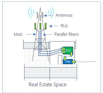
Figure 9: Cell site illustration for the DRAN fiber abundance case.
