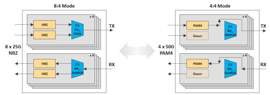
Currently, optical modules such as 200GE LR4 and ER4 of HiSilicon Optoelectronics support PAM4/NRZ mode switching on the electrical port side to meet the requirements of different application scenarios.
