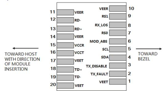
Figure 2 MSA compliant connector
