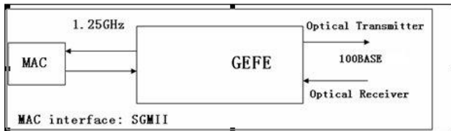
Figure 1. MAC to Fiber Connection
