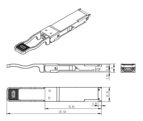
Figure 3. Mechanical Dimensions
