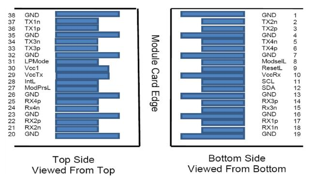
Figure 1. QSFP28-compliant 38-pin connector
