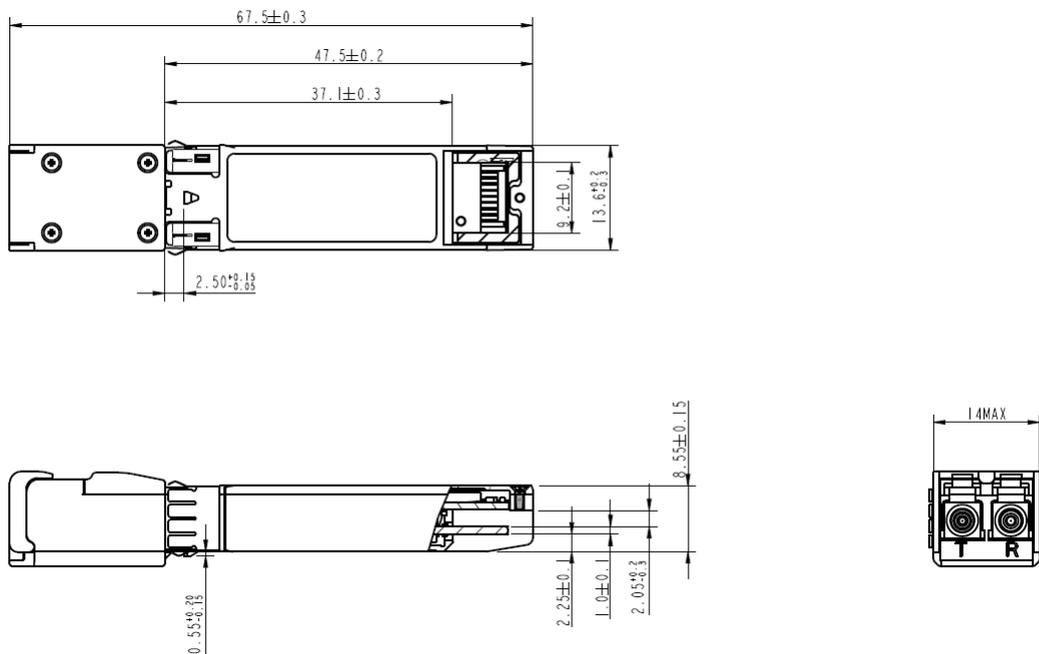
**Figure 3 Mechanical dimensions**
